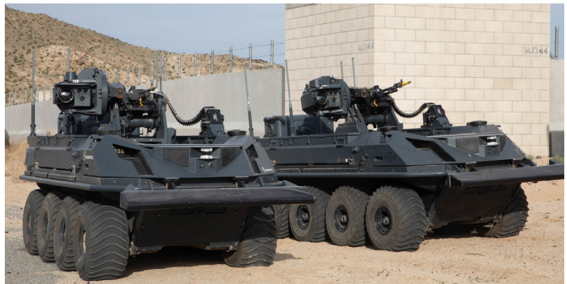
British unmanned, eight-wheeled, all-electric, transport vehicles armed with autonomous weapon system from the Experimentation and Trails Group provide support to dismounted U.K. Soldiers in an urban environment at Fort Irwin, Calif, March 11, 2024. (Image Credit: U.S. Army/Pfc. Ivan Hernandez)
